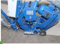
2. Floors and screeds must also be shot blasted or grinded to roughen the surface and produce an open pored, absorptive surface.
