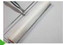
14. 4. Immediately after smoothing the material should be de-aired with a spiked roller. Spiked shoes must be worn during application while walking over the fresh material
